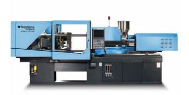
The electrical injection moulding machine, IntElect smart – here the model with a clamping force of 1,000 kN. Since the K 2010 it has been available with a clamping force of up to 4,500 kN and now a version with a clamping force of 1,600 kN can be seen at the Interplastica.
