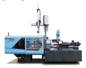
The integrated three-axis SDR robots are fully integrated in the NC5 control of the injection moulding machines made by Sumitomo (SHI) Demag and offer the customers of this producer of machinery a large product variety for factory-set automated injection moulding systems.
