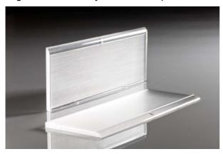
Light-conducting element made of PMMA, produced on a hydraulic injection moulding machine Systec 160-600 by means of the IMD method at the exhibition stand of Sepro Robotique, unloaded from the mould made by HBW-Gubesch by means of an integrated Demag Robot SDR 33.
