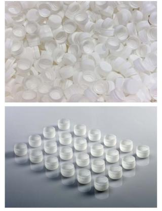
Lightweight caps made of HDPE with a tamper-resistant tape, injection moulded in a cycle time of less than 2.5 seconds on a high-speed injection moulding machine EI-Exis SP 300 made by Sumitomo (SHI) Demag in a 72-cavity mould made by KTW. Photograph: Sumitomo (SHI) Demag
