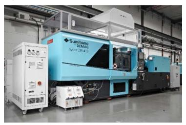
Compact production cell with a Systec 210, that combined IML and IMD technologies. This efficiently produces a multitouch display in a single machine.
