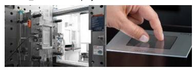
The frame of the 5" display is decorated on the moving half of the mould with the IMD unit directly during injection moulding.
