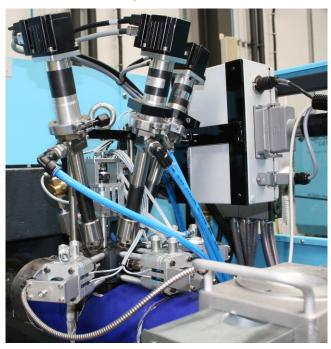
activeColourChange (for three colours) allows direct feed of liquid colorants into the metering zone of the plasticizing system; this new concept leads to a significant reduction in colour change times.
