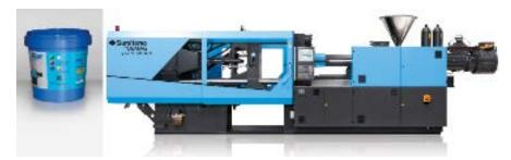
An IML decorated 1 I bucket, produced in a very efficient way using the new Systec SP 280 packaging machine with a cycle time of 5.3 s and a two-cavity mould.
