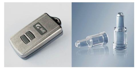
Products manufactured with all-electric IntElect precision: Smart key shell (on the left) with components made of PC/ABS blend, produced in a 6-cavity family mould on an IntElect 100, and components for a "Braunüle" (on the right), made of MABS and under cleanroom conditions on an IntElect 50.
