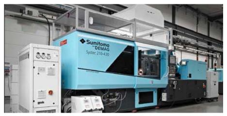
Compact production cell with a Systec 210 combining IML and IMD technology. A multitouch-capable display is produced here in one shot.
