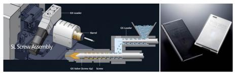
Parts of a smartphone housing made of an ABC/PC blend using an all-electric SE 180 EV which is equipped with the modern SL plasticising assembly. The assembly operates with a completely heated screw without a compression zone (screw); the material is fed by an upstream dosing screw (GS Loader).
