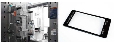
On the clamping side of the mould the frame of the 5" display is decorated using the IMD unit directly during injection.
