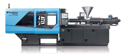
The Systec machines available from 350 to 20,000 kN represent an economical production solution for the broad range of standard applications. At the Interplastica, a 2,100 kN version will be producing the lower portion of a coin dish made from polystyrene Photo: Sumitomo (SHI) Demag
