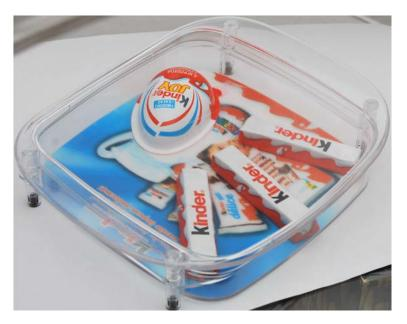
Lower portion of a coin dish made from polystyrene on a Systec 210-840 hydraulic injection moulding machine using a mould from Viki Vostok.
