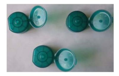
Flip-tops, manufactured on an all-electric IntElect 220-1100 injection moulding machine in a 12-cavity mould from GIFLOR Srl
