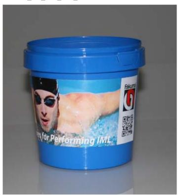
The 1 I buckets made of PP are produced using a twocavity mould on the hybrid El-Exis SP 250 (2,500 kN) high-performance machine in a cycle time of under 4.5
