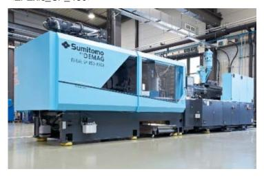
An El-Exis SP 250, in this case a model with a 4,500 kN closing force, will be at the trade show. It will be demonstrating the capabilities of a high-speed production unit for manufacturing buckets, associated with a new speed side-entry from Sepro Robotique.
