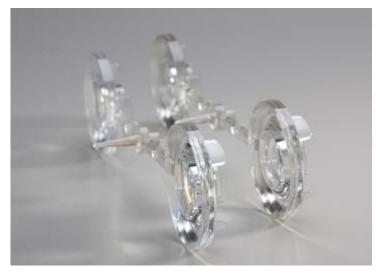
Thick-walled precision lenses are produced on the gwk stand using a fully electric IntElect 100: due to a new mould concept, the influence of the applied cooling process can be rendered directly comparable. Photo: gwk
