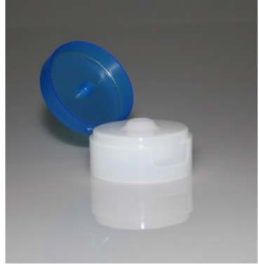
The 2-component fliptop is produced in groups of 16 on an IntElect multi in fewer than 14 seconds. It is closed by means of a function integrated in the mould before being ejected, in order to reduce the follow-on steps. Photo: Sumitomo (SHI) Demag
