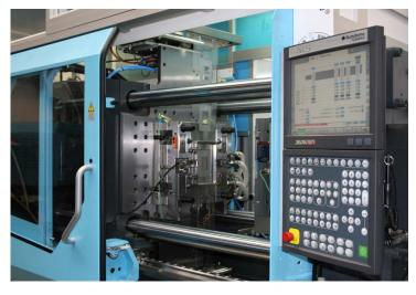
The Systec 210 multifunction machine will feature a highlight at Fakuma 2012: a compact production unit combines IML for the function foil and IMD for the surface decoration, to produce a 3.5-inch display control panel.
