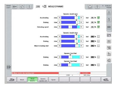
New activeAdjust function: Using a slider, the operator can increase or – if required – decrease the dynamics of the mould movement to suit the individual application, without external help. Photo: Sumitomo (SHI) Demag
