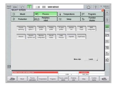
By consistently dividing all functions into primary and secondary groups, each screen can be called up with a maximum of two clicks; this eliminates having to call up screen lists and then having to scroll through them. Photo: Sumitomo (SHI) Demag
