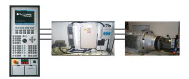
The variable-speed smartDrive pump drive gives the user an economical solution, because it is sufficient to connect a frequency converter on the supply side of the asynchronous pump drive motor to allow the motor's speed to be controlled.
