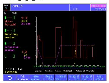
According to the particular user settings, smartDrive adjusts the motor speed automatically to the requirements of the particular cycle, and only provides the power that the machine actually needs in each cycle sequence. When there are length rest phases in the cycle, this also reduces overall consumption because higher percentage savings are available during these phases.
