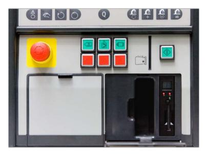
The CompactFlash retrofit kit replaces the floppy disk drive.
