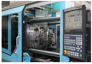
The Systec 210 multifunction machine will feature a highlight at the Fakuma 2012: a compact production unit combines IML for the function foil and IMD for the surface decoration, to produce a 3.5-inch display as a control panel.
