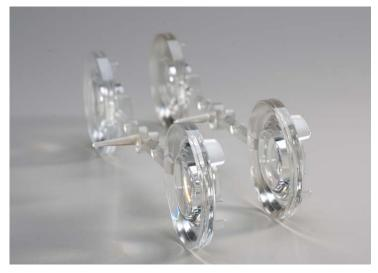
Thick-walled precision lenses are produced on the gwk stand using a fully electric IntElect 100; due to a new mould concept, the influence of the applied cooling process can be rendered directly comparable. Photo: Sumitomo (SHI) Demag
