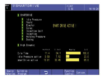
By using a variable-speed pump drive, it is possible to reduce the energy consumption of hydraulic injection moulding machines considerably; the measure, under the heading of smartDrive, can even be retrofitted to older machines
