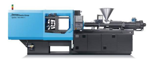
The energy-efficient hydraulic Systec C injection moulding machines produced by Demag Plastics Machinery (Ningbo) – in this case a Systec 160-840 C
