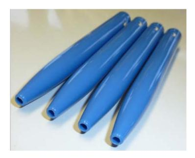
Ball point housings made on an all-electric injection moulding machine IntElect 100-430 on a four-cavity mould made by Werkzeugbau Ruhla GmbH
