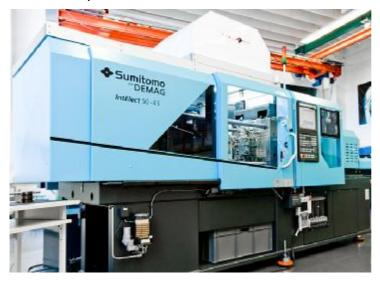
The all-electric injection moulding machine IntElect 50-45 made by Sumitomo (SHI) Demag with a clamping force of 500 kN – Figure shows a model configured for the cleanroom production of medical precision mouldings Photograph courtesy of Sumitomo (SHI) Demag
