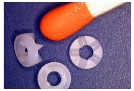
Control knob made of POM for hearing aid devices, made on an all-electric injection moulding machine IntElect 50-45 in the cleanroom on a four-cavity mould made by Stamm AG Photograph courtesy of Stamm AG
