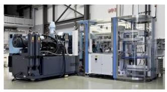
The compact production cell for Full Cover Labelling consists of a hybrid El-Exis SP 200 high performance machine (left) as well as a Full Cover Label Placer from Marbach (right)
