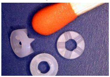
Control knob made of POM for hearing aids, manufactured on an all-electric IntElect 50-45 injection moulding machine in a clean-room in a 4-cavity mould of Stamm AG
