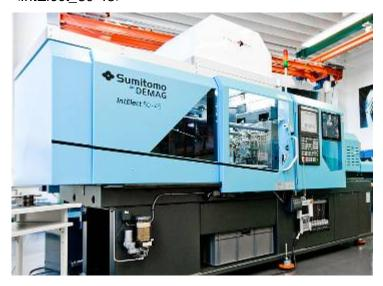
The IntElect 50-45 all-electric injection moulding machine from Sumitomo (SHI) Demag with 500 kN clamping force – here with equipment for the clean-room production of medical precision parts.
