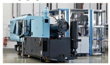
Hybrid high-performance cell built around an El-Exis SP 200 with IML automation and IML mould from Marbach for full-cover labelling
