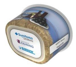
Full-cover labelling is the name if the new in-mould labelling process from Marbach. For this process, the banner label and the base label are inserted overlapping around a radius, thereby providing complete coverage of the plastic surface with the label up to a high level on the sealing edge.
