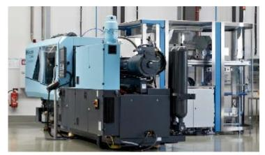
Hybrid high-performance cell built around an El-Exis SP 200 with IML automation and IML mould from Marbach for full-cover labelling.
