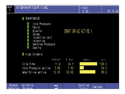
By using a pump drive controlled by rotational speed (activeDrive), the energy consumption of hydraulic injection moulding machines can be considerably reduced; the feature is also available under the name "smartDrive" as a retrofit for older Systec machines.
