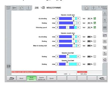
New activeAdjust function: Using a slider, the operator can increase or – if required – decrease the dynamics of the mould movement to suit the individual application, without external help.
