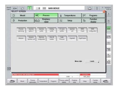
By consistently dividing all functions into primary and secondary groups, each screen can be called up with a maximum of two clicks; this eliminates having to call up screen lists and then having to scroll through them.
