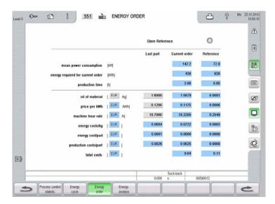
The new activeEcon function offers the user not only built-in energy measurement and analysis of energy consumption, but also direct monitoring of production costs by taking into account the costs of materials and electricity, as well as the machine hourly rate.
